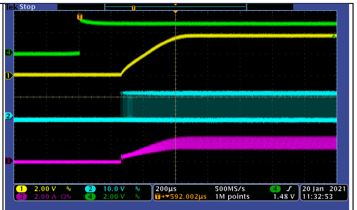
Fig 8 Enable Start up (Vin=12V, Vout=3.3V, I LOAD =2A)
